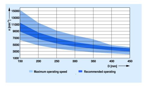
Figure 12: Speed n as a function of circular saw blade diameter D (source: Leitz GmbH & Co. KG)
