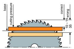
Figure 7: Correct saw blade projection for fixed circular saws and sliding table saws (source: Leitz GmbH & Co. KG)
