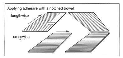
Figure 21: Applying adhesive
