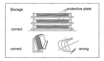
Figure 3: Correct storage of laminate sheets
