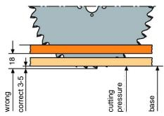
Figure 6: Correct blade projection for portable circular saws with plunge function (source: Leitz GmbH & Co. KG)
