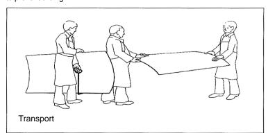
Figure 4: Correct handling of laminate
