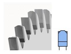
Figure 10: Trapezoidal / flat tooth (source: Leitz GmbH & Co. KG)
