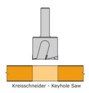
Figure 17: Hole saw (source: Leitz GmbH & Co. KG)
