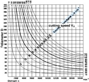
Figure 18: Cutting speed as a function of rotational speed and tool diameter (source: Leitz GmbH & Co. KG)
