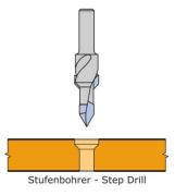
Figure 15: Multi-diameter/step drill (source: Leitz GmbH & Co. KG)
